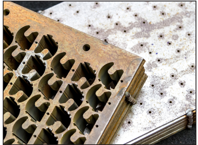
Milco speeds part production using "stack ups" – raw pieces of material cut on its OMAX waterjets, stacked together, tack welded in place, then wire EDMed from start holes also cut with on waterjet machines
