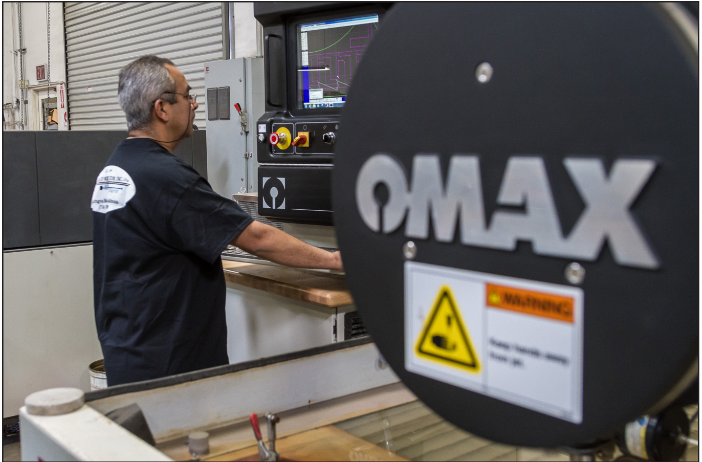
Cutting near-net shaped part blanks on OMAX waterjet machines helps reduce part costs at Milco because there's less raw material involved.
